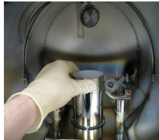
Upper Left: Removal of Filament Shield
