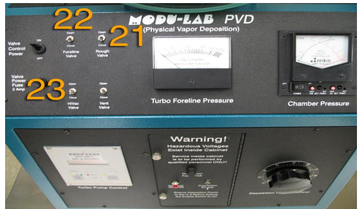
Above: Switches corresponding step number. High Vacuum pumps down from 10^{-1}-10^{-5}\text{mTorr}
