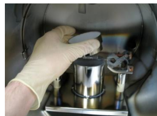
Upper Left: Replacing Filament Shield
