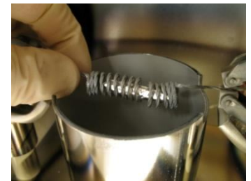
Upper Left: Replacing loaded Filament into screw clamps
