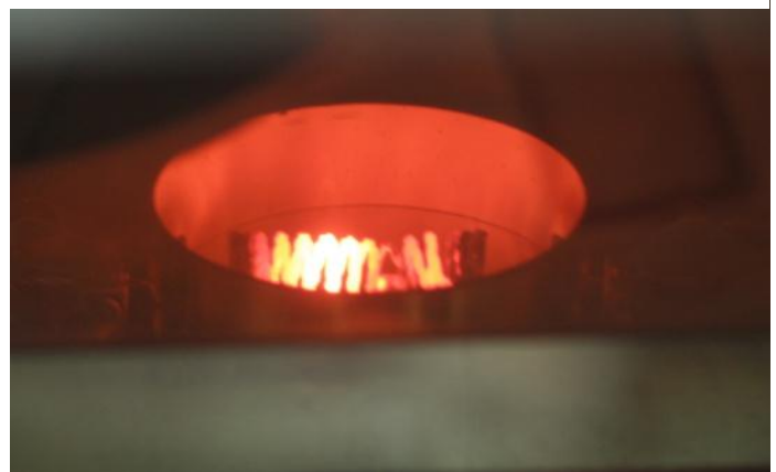
Above: Aluminum sample begins to melt at DPC = 40%
