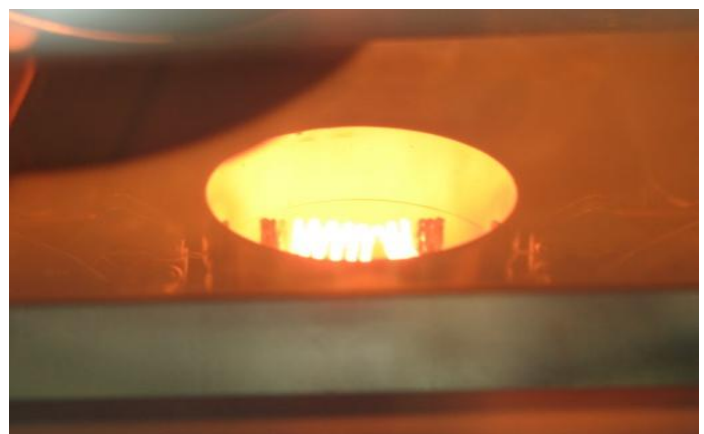
Above: Aluminum sample evaporates at DPC = +60%
