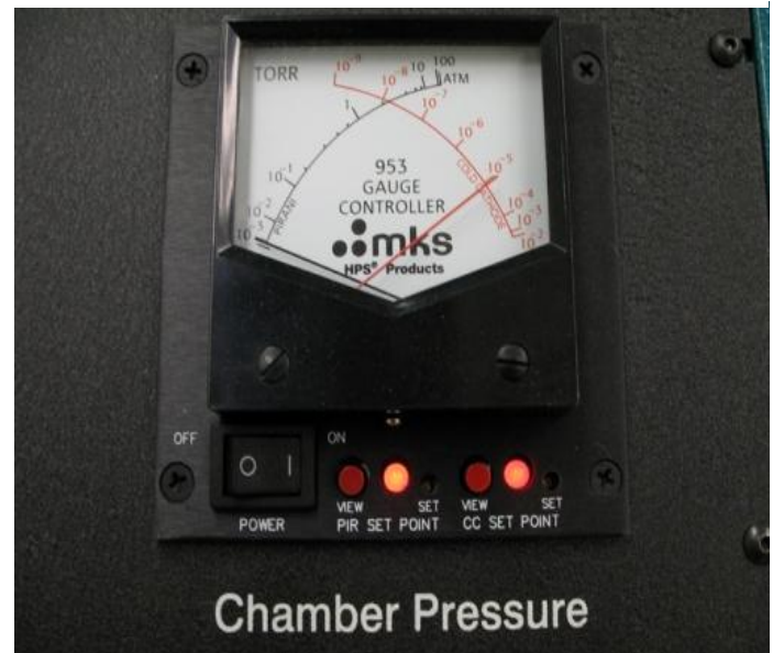
Above: Chamber Pressure (Cold Cathode) reads \sim 10^{-5}\text{mTorr} , Ready for deposition
