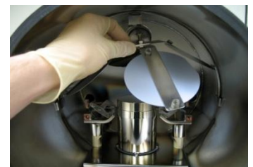
Upper Left: Replacing Filament Shield
