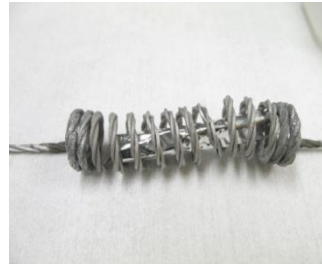
Upper Left: Aluminum evaporation sample loaded into Filament
