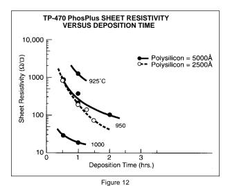
Doping Properties of PhosPlus Sources. Uniformities: When the various processing conditions are optimized, uniformities of 2% across the silicon, 3% across the boat and 4% run-to-run or better can generally be obtained on single-crystal silicon. A total variation of about 3% can be achieved on high-quality polysilicon wafers doped to their minimum sheet resistivities (saturation with phosphorus).
