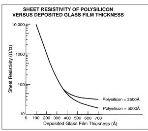
■ Doping Properties of PhosPlus Sources. Polysilicon: The minimum sheet resistivity that can be obtained from polysilicon wafers that are saturated with phosphorus partially depends upon the thickness of the polysilicon layer as shown in Figure 9. These sheet resistivities are about  $12 \Omega/\Box$  for 5000Å of polysilicon and about  $32 \Omega/\Box$  for 2500Å, and they occur when the deposited phosphorus glassy film exceeds about 500 to 600Å as shown in Fig. 10.
