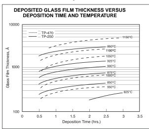
A typical deposition time for a solid-source diffusion system is about 45 minutes. This time is usually long enough for the sources to uniformly dope the silicon wafers. At the same time, it is short enough to be compatible with most semiconductor process parameters. Figure 8 shows the sheet resistivity and junction depth that is obtained from a 45-minute deposition with the TP-470 PhosPlus sources at various deposition temperatures.
