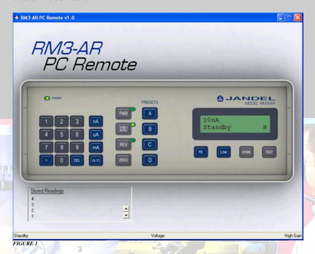
Note that the LED's are also represented. In figure 1 the unit is in 'standby' and so the LED next to the standby button is illuminated.
