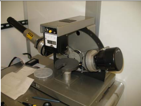
Figure 8 The oxide thickness is measured using the ellipsometer. It measures the light intensity as a function of polarization reflected off the surfaces on the wafer
