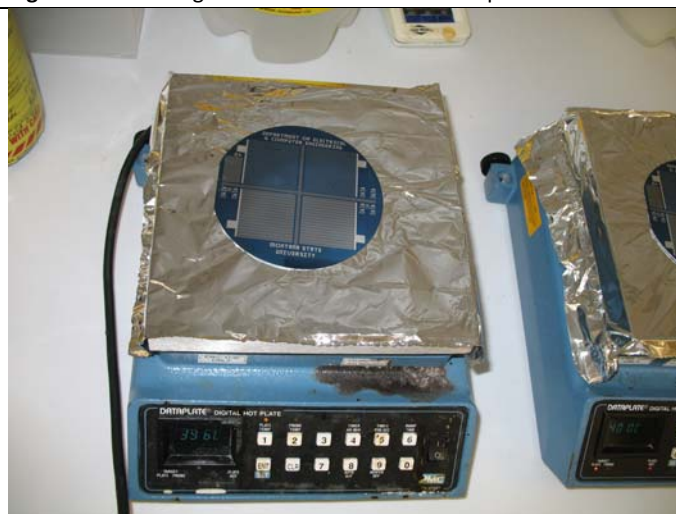
Figure 20 Annealing the solar cell wafer on a hot plate.
