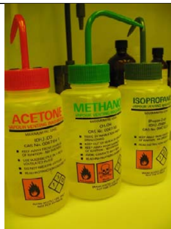
Figure 10 Use a three solvent clean to remove the photoresist from the wafer.
