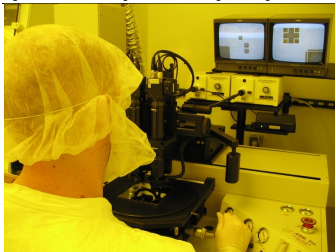
Figure 17 A student using the ABM mask aligner to align Mask #3.
