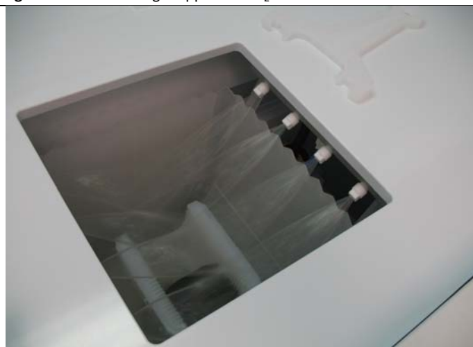
Figure 12 Wafers being stripped of SiO 2 in a 6:1 BOE solution.
