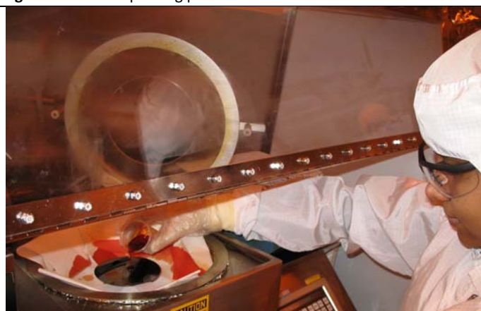
Figure 15 Student pouring photoresist on wafer .
