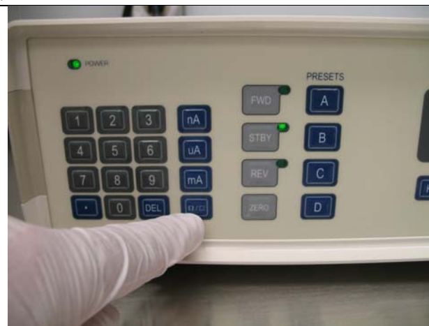
Figure 7 The sheet resistivity measurement is taken by pressing the ' \Omega/\square ' button.
