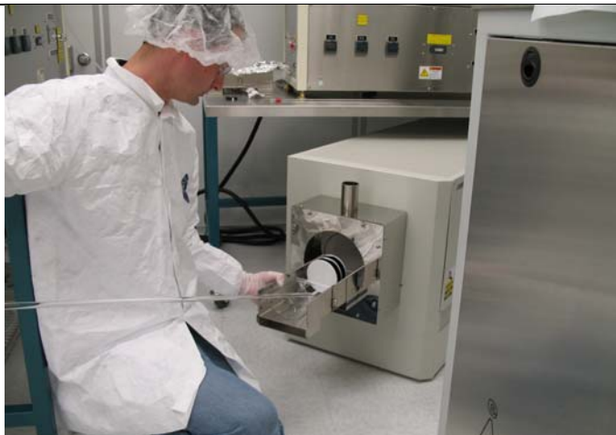
Figure 5 Inserting the boat into the Boron Diffusion Furnace.
