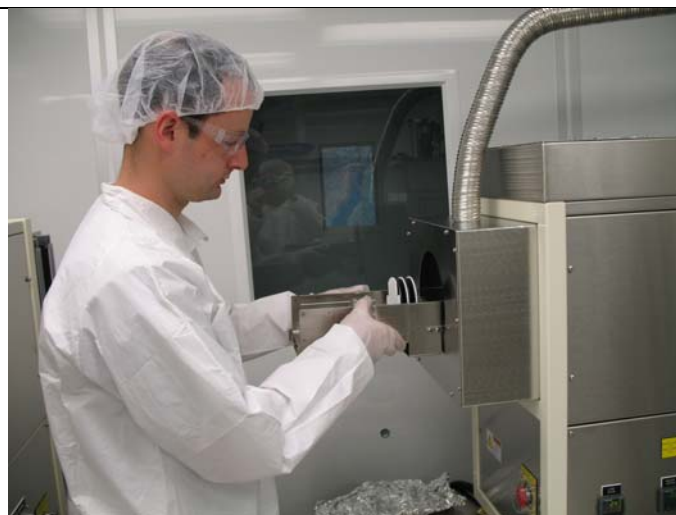
Figure 13 Placing the boat tray on the front of the Phosphorus Diffusion Furnace .
