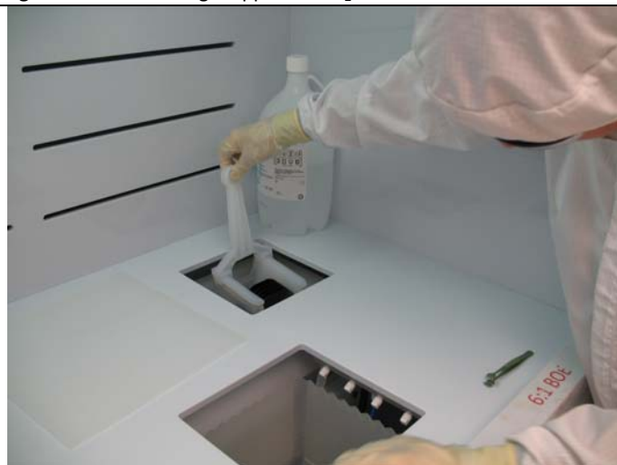
Figure 11 Wafers being stripped of SiO 2 in a 6:1 BOE solution.
