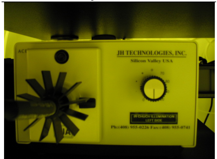
Figure 25 The infrared light sources used for backside alignment located beneath the mask aligner
