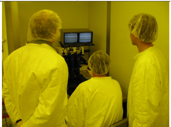
Figure 23 Students and professor looking on as a wafer is aligned and exposed at the ABM contact aligner.
