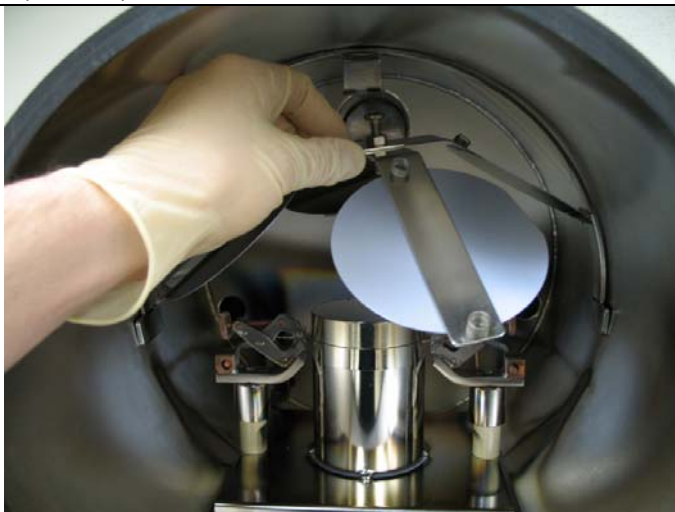
Figure 22 Wafers being loaded into the aluminum physical vapor deposition system.
