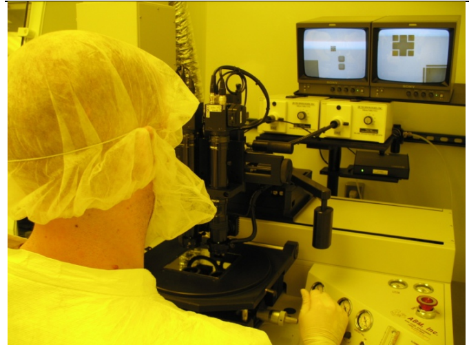
Figure 45 A student using the ABM mask aligner to align Mask #7.
