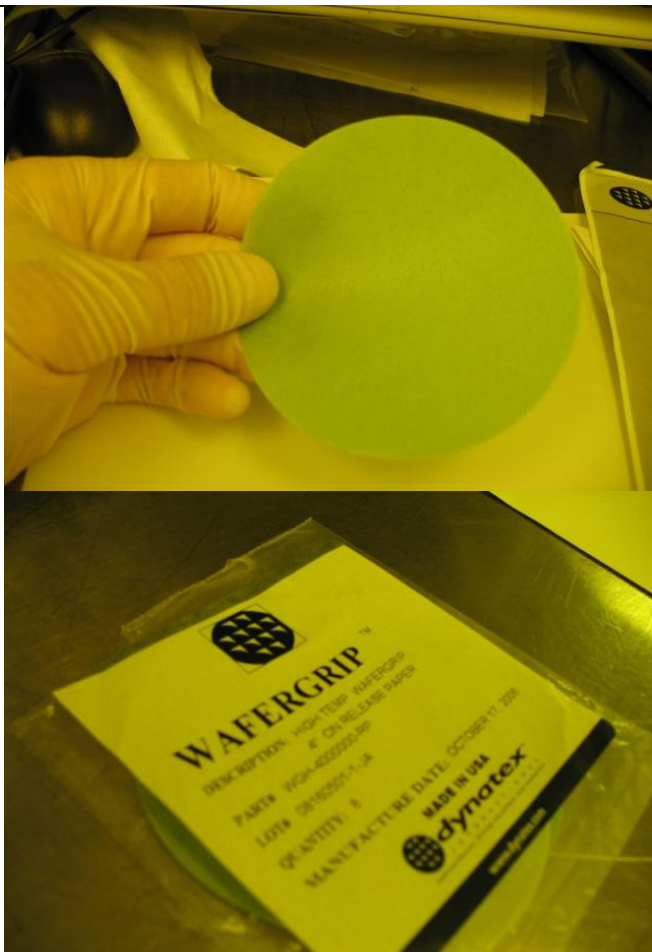
Figure 40. The WAFERGRIP adhesive used for the temporary wafer bonding.
