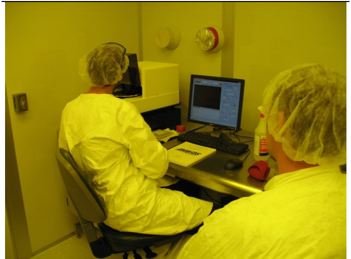
Figure 31 Two students operating the AMBIOS profilometer to monitor the etch depths of the bulk silicon etch.
