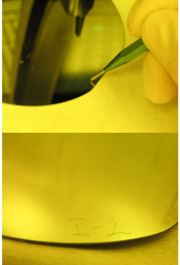
Figure 4 A student using a quartz rod to insert wafers into the oxidation furnace.
