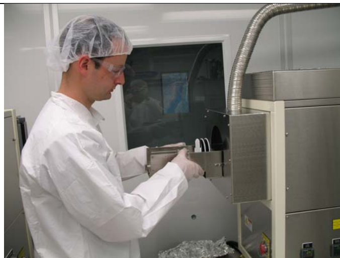
Figure 7 Placing the boat tray on the front of the Phosphorus Diffusion Furnace .
