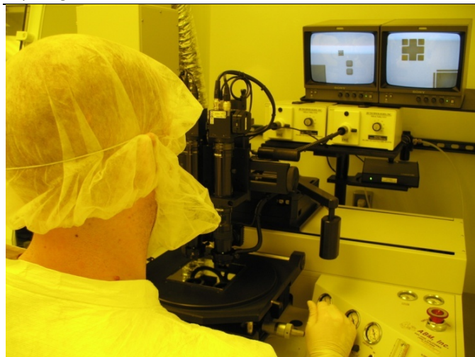
Figure 14 A student using the ABM mask aligner to align Mask #3 and exposing.
