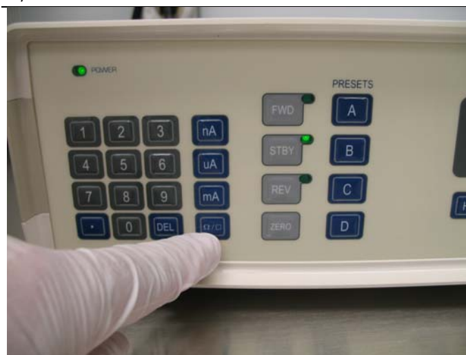
Figure 19 The sheet resistivity measurement is taken by pressing the 'Ω/□' button.
