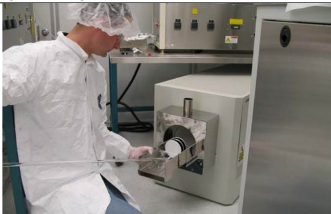
Figure 5 Inserting the boat into the Boron Diffusion Furnace.
