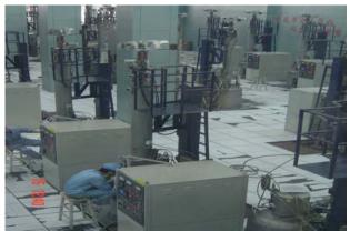
Figure 14: Cz crystal pullers growing single-crystal ingots
