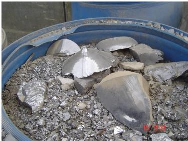
Figure 26: A drum of scrap silicon chips awaiting re-melting and growth into <u>ingots</u> for later sawing into wafers for solar cell manufacture
