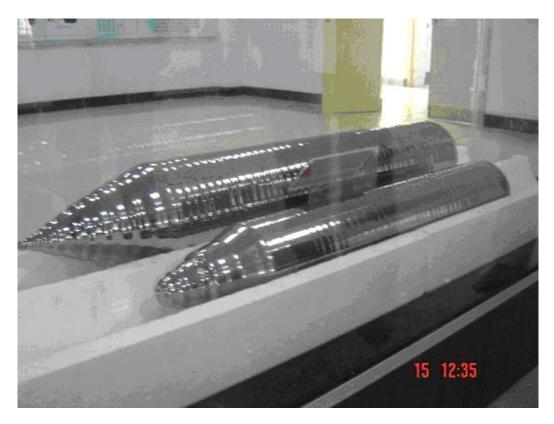
Figure 9: Silicon <u>ingots</u> prior to sawing into wafers. Each ingot is a single crystal (Photo courtesy of Dr. R. Corkish)
