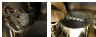
Upper Left: Replacing loaded Filament into screw clamps Upper Right: Close-up of ridges on screw clamps
