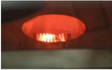
Above: Aluminum sample begins to melt at DFC = 40%
