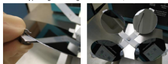
Upper Left: Close-up of a spring clip Upper Right: Fully-loaded Wafer Holder
