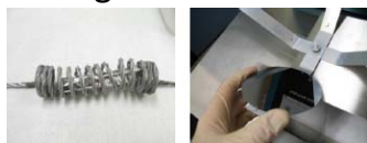
Upper Left: Aluminum evaporation sample loaded into Filament Upper Right: Loading a wafer into Wafer Holder
