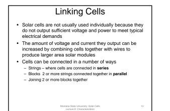
Solar Cell Panels Current Current Parallel connections increase the current output Voltage Voltage Blocks Series increase connections both current Curren increase the and voltage voltage output output Voltage a State University: Solar Cell cture 8: Characterization
