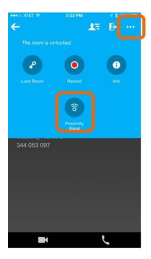
The proximity application is cross launched with the video address of the WebEx meeting. You can now control the TelePresence unit or video device with the Proximity application on your mobile device.
