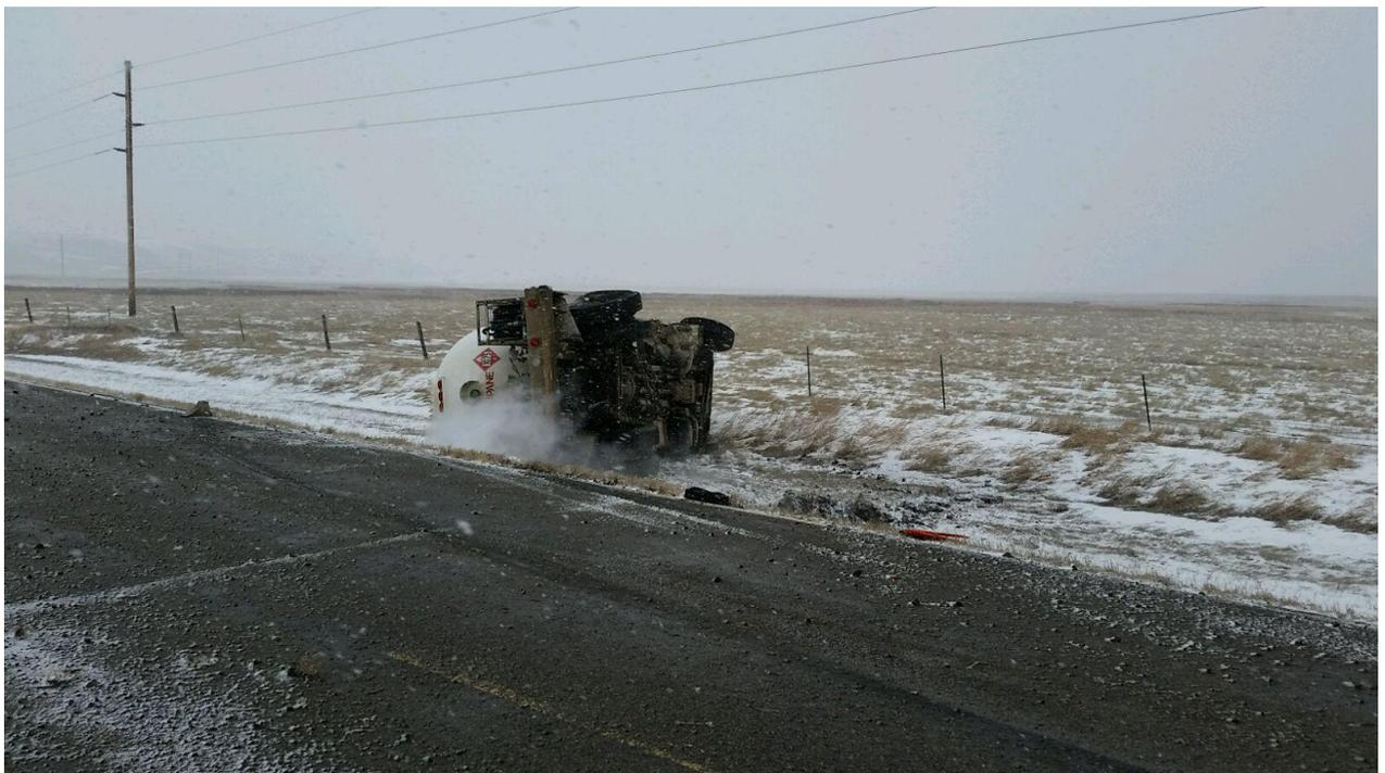
When the truck wrecked, it caused a propane leak from a valve. It was estimated to be leaking 2-4 lbs. a minute. Estimated loss was 955 lbs. They were able to transfer 2,700lbs. into other propane trucks. It took about 6 hours to do that.
