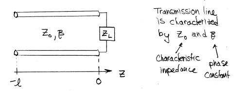
Recall that the reflection coefficient at the load is given by  $\Gamma_L = \frac{Z_L - Z_0}{Z_L + Z_0}$ . Now however we seek the reflection coefficient at an arbitrary point on the transmission line.
