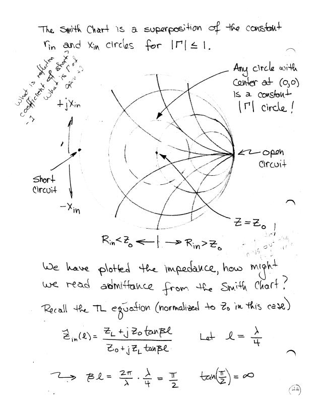
$\vec{z}_{in}(l=\frac{1}{4}) = \frac{z_{L}+jz_{0}(\infty)}{z_{0}+jz_{L}(\infty)} = \frac{z_{0}}{z_{L}} \rightarrow$ ЧL Thus we can determine  $\hat{y}_{L}$  by rotating  $\frac{\lambda}{4}$ from  $Z_{L}$ . constant [1] circle Ì 4L 1/4 Recall that M and Zin repeat every 1/2 which is one complete revolution on the Smith Chart.
