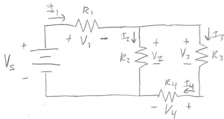
$$\text{Loop 1: } V_s - V_1 - V_2 = 0$$
