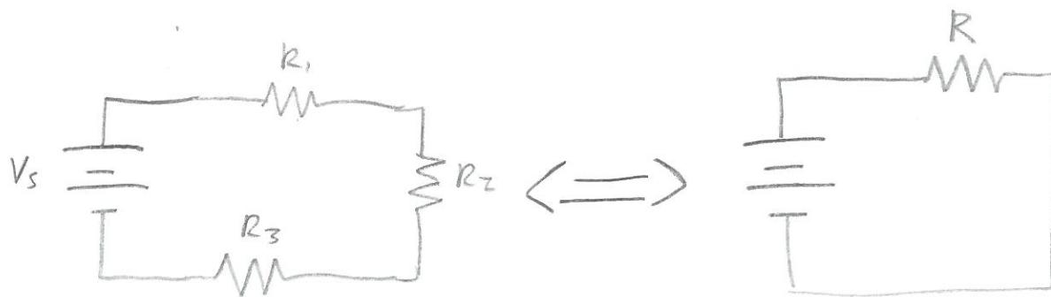
From the perspective of the battery, total resistance in the circuit is  $R = R_1 + R_2 + R_3$
