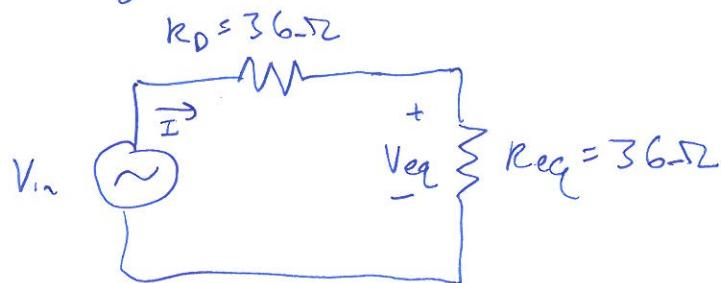
$$I = \frac{V_{in}}{R_D + R_{eq}} = \frac{120V}{72\Omega} = 1.67A$$
