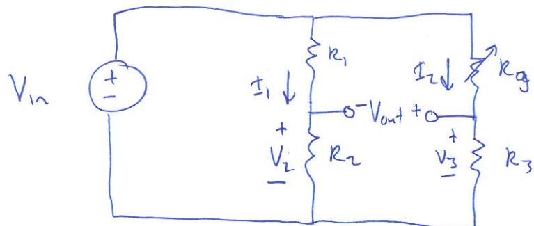
→ Label currents through each branch as  $I_1$  and  $I_2$ , and voltages across branch  $R_3$  as  $V_3$  and  $V_2$ , respectively.
