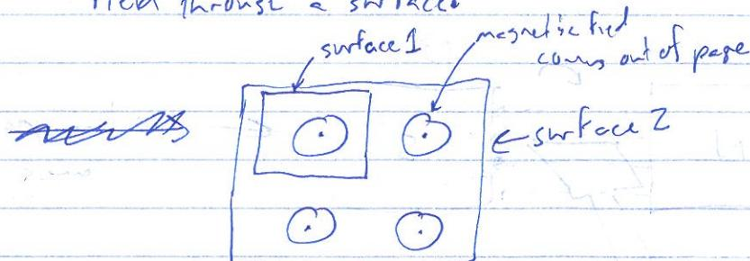
Larger area means greater magnetic flux as there are more magnetic field lines passing through it.
