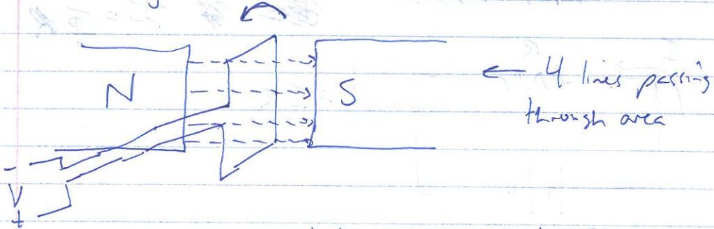
As the loop rotates, the magnetic flux through it changes because the surface of the loop rotates so that the number of magnetic field lines through the loop changes.
