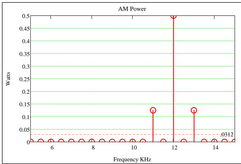
$f_m = 1 \text{ KHz}$  Modulating frequency
