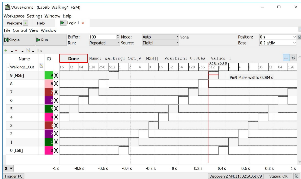
Figure 9.13 Logic Analyzer Measurement of Walking 1 Pattern
