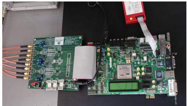
**Figure 4. A/D board connected to the FPGA platform.**
