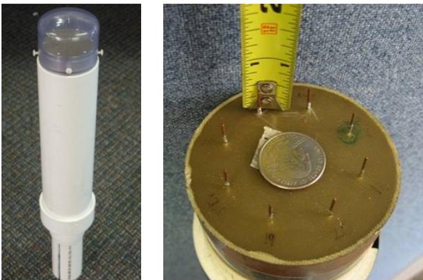
**Figure 2. 5.8GHz circular antenna head.**
