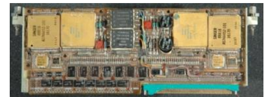
Precedent: Shuttle Flight Computer (TMR + Spare)
