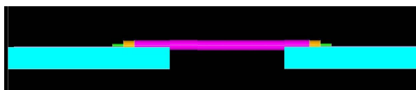
Figure 1. Side View of the Proposed Interconnect System Connecting Two Adjacent Dies.
