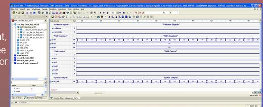
When radiation is detected by the external sensor (radiation), the system enables the two redundant counters (en2, en3) and loads them (load2, load3) with the current count value (in1). During this time, the system output pauses (pc\_out) to accommodate the start-up time of the two redundant counters.
