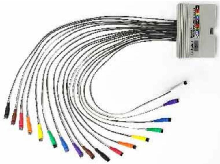
This is different from previous flying lead sets in which one ground could be used across all 17 channels. The reason for this constraint is to enhance the performance of the probe. The figure above shows an example of a differential flying lead probe.
