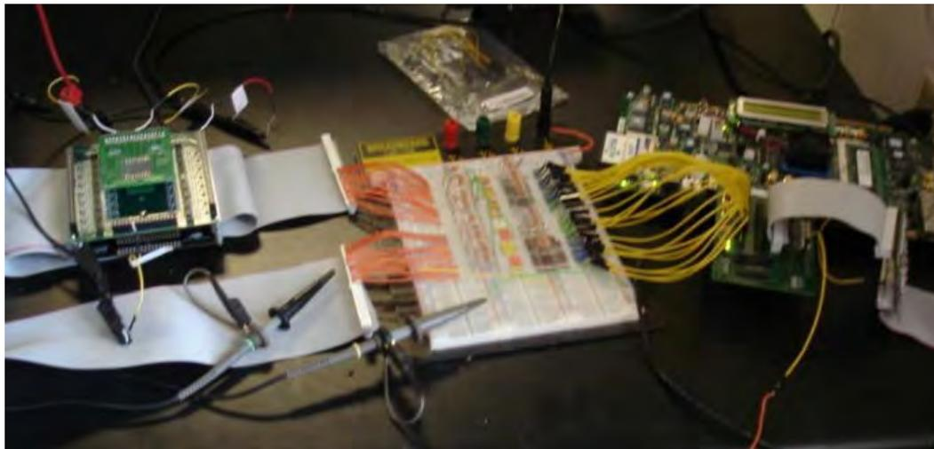
Figure 3-2. Breadboarded prototype of the RTCS.
