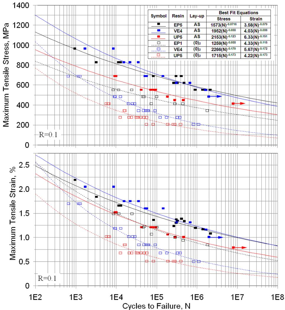
Figure 6. Comparison of stress and strain fatigue trends for aligned strand and (0)<sub>2</sub> fabric H based laminates for epoxy (EP1 and EP5), vinyl ester (VE4) and polyester (UP5) resins.
