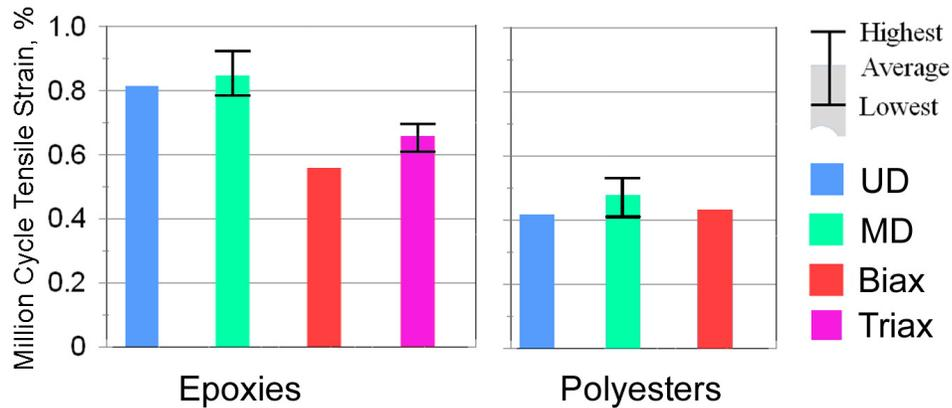
Figure 3. Comparison of million cycle fatigue strains for typical EP and UP resin laminates.
