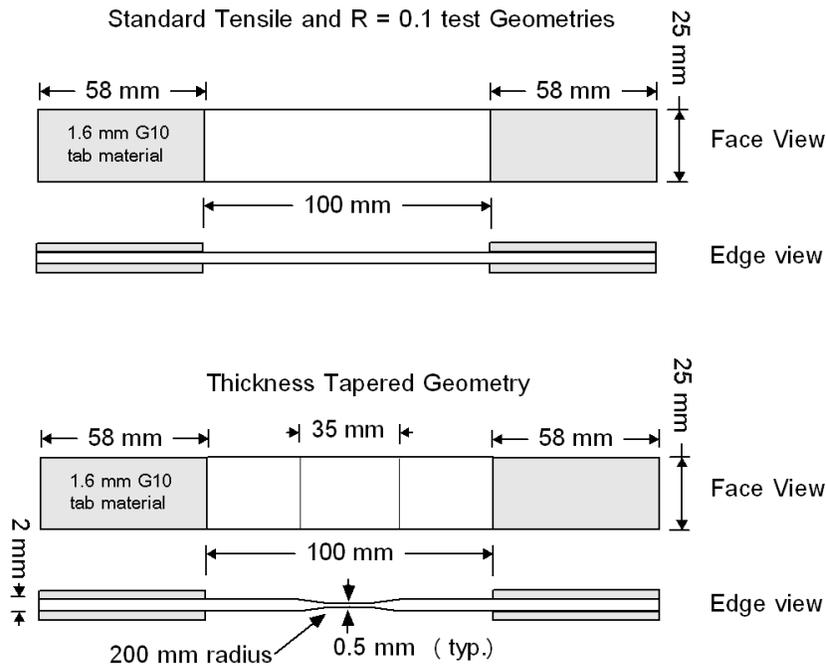
**Figure 2. Standard (top, 2-mm thickness) and thickness tapered tensile fatigue coupons for UD laminates.**
