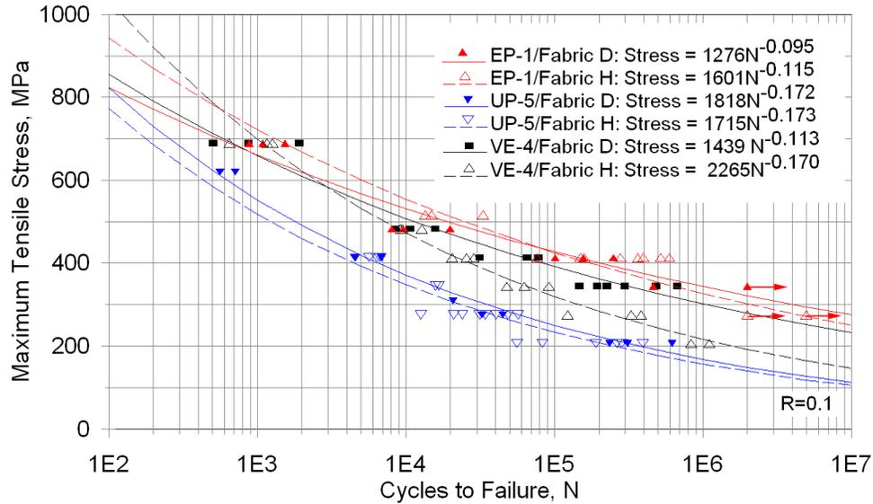
Figure 7. Effect of UD fabric D vs. fabric H, for EP, VE and UP resins, (0)<sub>2</sub> laminates.
