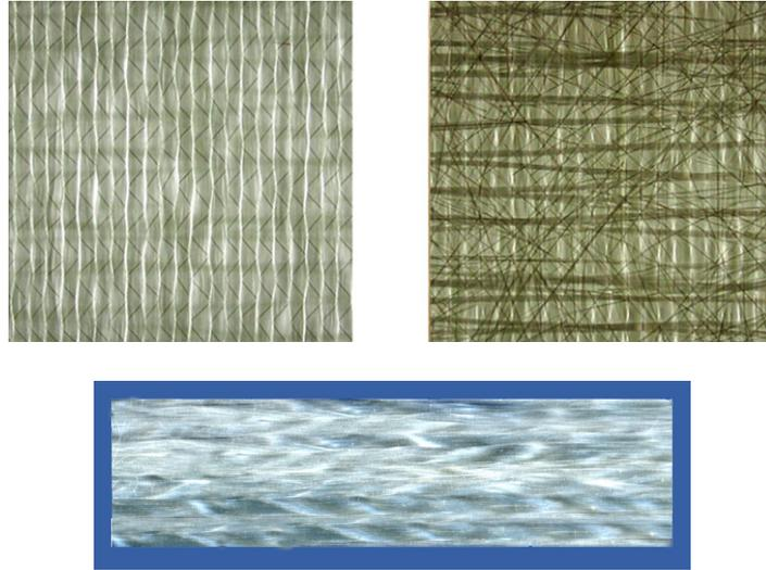
**Figure 1. Top: front and back views of UD fabric H; bottom: aligned strand structure.**
