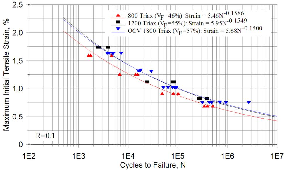
**Figure 10. Strain vs. cycles to fail for triax fabric laminates with two Saertex fabrics (800 and 1200 gsm) and a heavier OCV™ fabric (1800 gsm), epoxy EP1, R = 0.1.**
