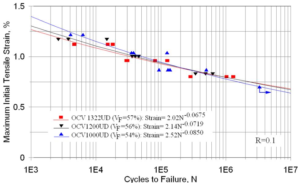
Figure 9. Strain vs. cycles for UD laminates with three different weight OCV™ fabrics, EP1 epoxy, R = 0.1.
