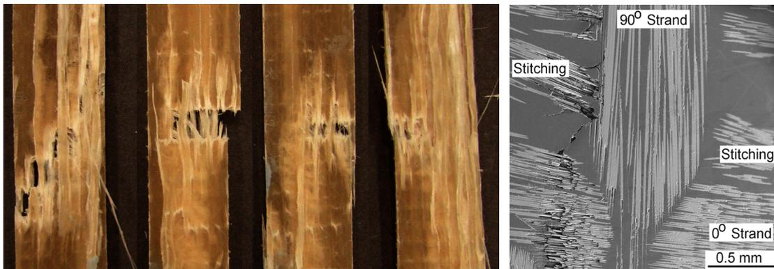
Figure 4. Cracking along transverse ( $90^\circ$ ) backing strands of UP5/fabric laminate; left: failed coupons; right: micrograph of crack following the backing strand, and failing the  $0^\circ$  strand.
