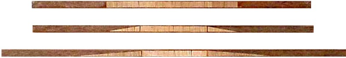
Figure 186. Thick Termination Specimens: 90 (top), 10 and 5 (bottom) Degrees.
