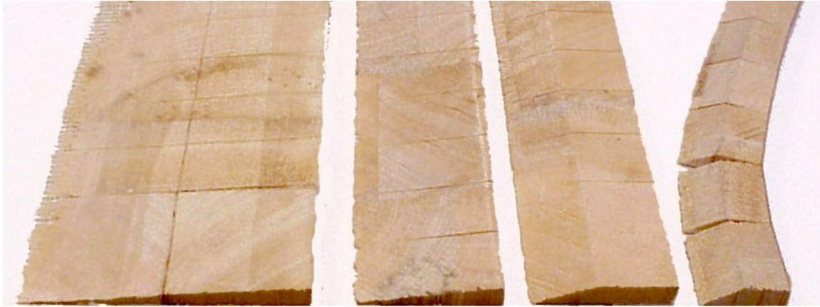
Figure 193. Balsa Fillet Strips for Various Tests (left to right): 5, 10, 20 and Baltek 30 Degrees.
