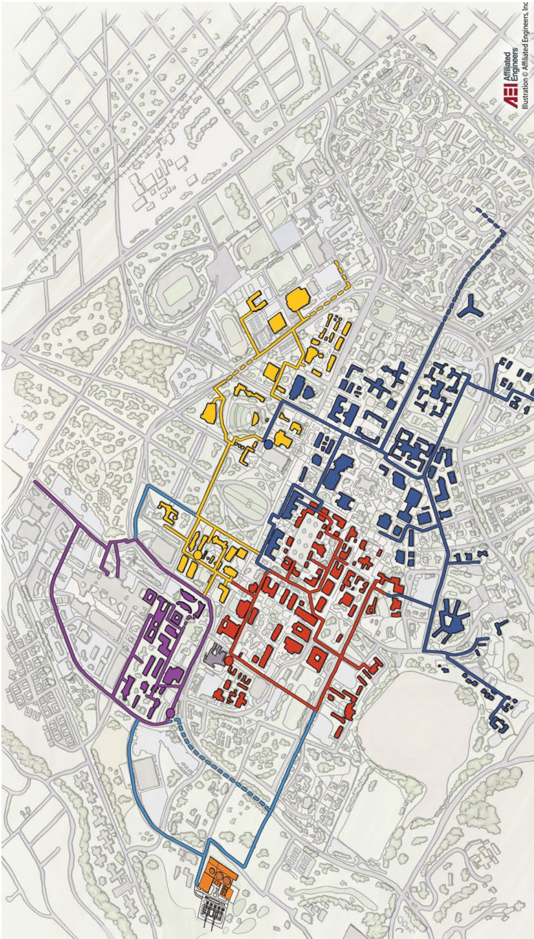
FIGURE 0-4 HOT WATER PIPING CONVERSION MAP
