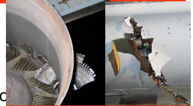
Rotor Disk Cut Through the Aircraft Fuselage Belly and Wing Center Section to Reach Opposite Engine
