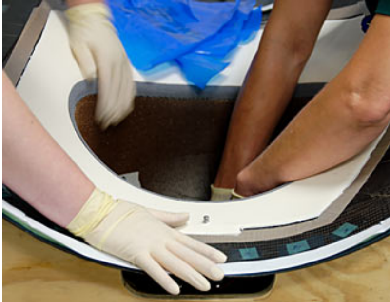
Figure 3. Example of Hand Lay-up Construction [12]
