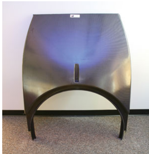
Figure 7. Complex, Net Shape Part made with Vacuum Assisted Resin Transfer Molding (VARTM) Processing [16]
