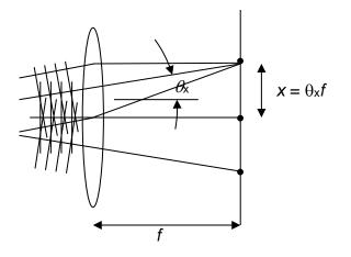
If the lens is placed behind the aperture in the previous arrangement we have the following relationship, after substituting for  $\theta_x = x/f$  and  $\theta_y = y/f$ :
