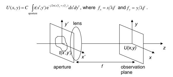
We will use these basic results to interpret the diffraction patterns produced in the lab.
