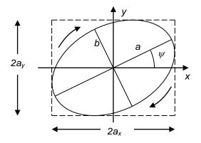
It is possible to use a local coordinate system to describe the ellipse in terms of its major axis component *a* and minor axis component *b*, along with the angle  $\psi$  that the major axis makes with respect to the laboratory *x* axis. The *ellipticity* of the polarization state is specified by *b/a*, and we call  $\psi$  the polarization angle. Note that the ellipticity is defined in terms of field amplitudes, so it can be calculated as the square root of the ratio  $I_{min}/I_{max}$ .
