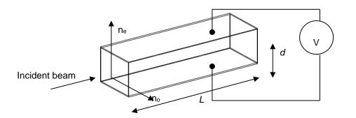
The electric field is applied along the vertical axis, which is the extraordinary axis of the crystal. In this case we can write for the ordinary and extraordinary indices of refraction:
