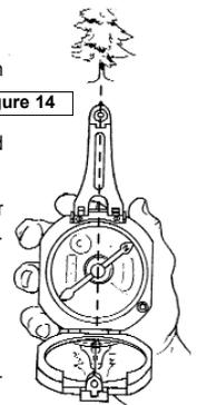
If object is more than 45° above you, open mirror further toward your body, and adjust large sight so that it leans over the bottom case. Then repeat the procedures described in 4.2.a.
