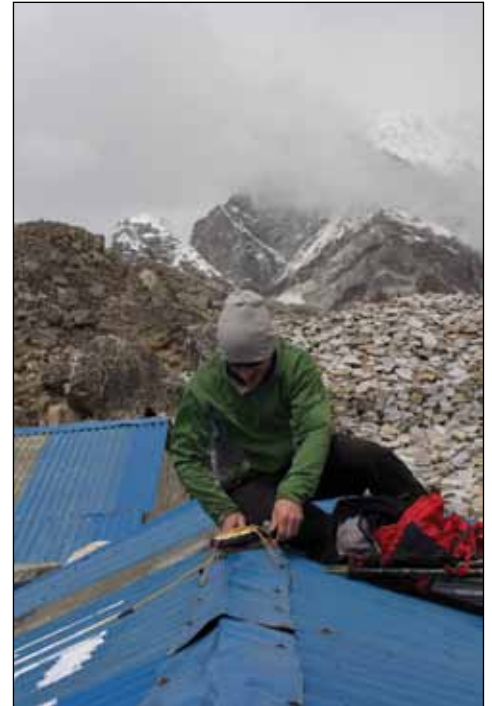
Travis adjusts the Trimble basestation antenna on top of the teahouse roof.
