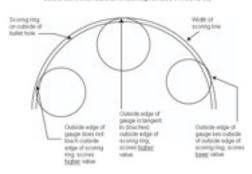
SCOBING WITH OUTWARD SCOBING GAUGES.
