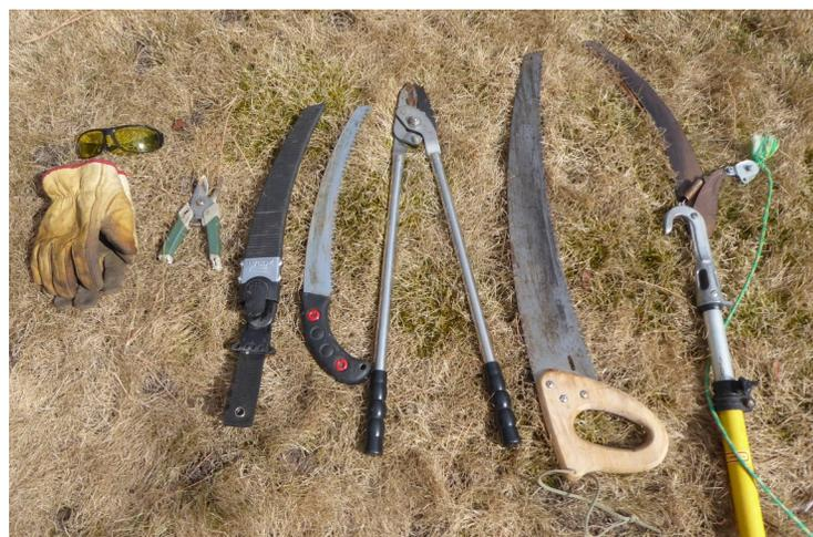
**Figure 2.** Pruning tools you will want are comfortable leather gloves, safety glasses, hand clipper, small pruning saw, lopper, a larger saw or small chainsaw, and a pole saw. Higher quality tools, but not always the most expensive, make the job easier.
