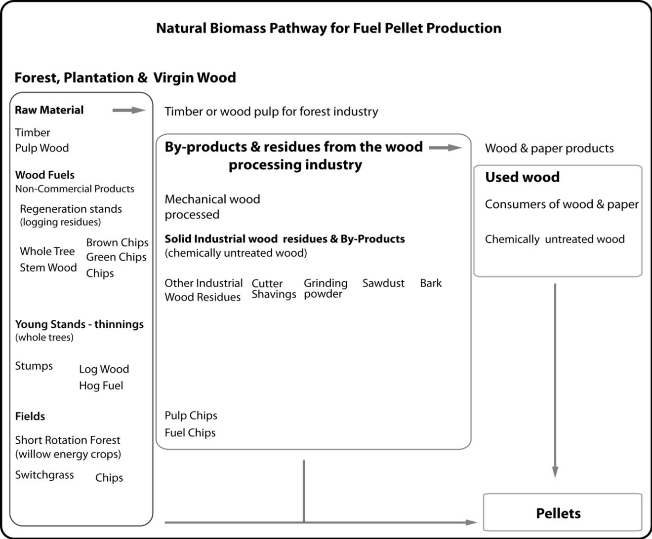
The diagram above describes the pathway for fuel pellet production. Along each pathway energy is used and emissions are created.
