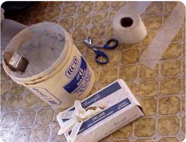
Duct mastic and self-adhesive fiber tape is easy and fast to apply, and is the very best duct-sealing solution. It sticks to everything, which is good -- but because it's so messy, you'll need rubber gloves, rags, and plastic to protect nearby surfaces.
