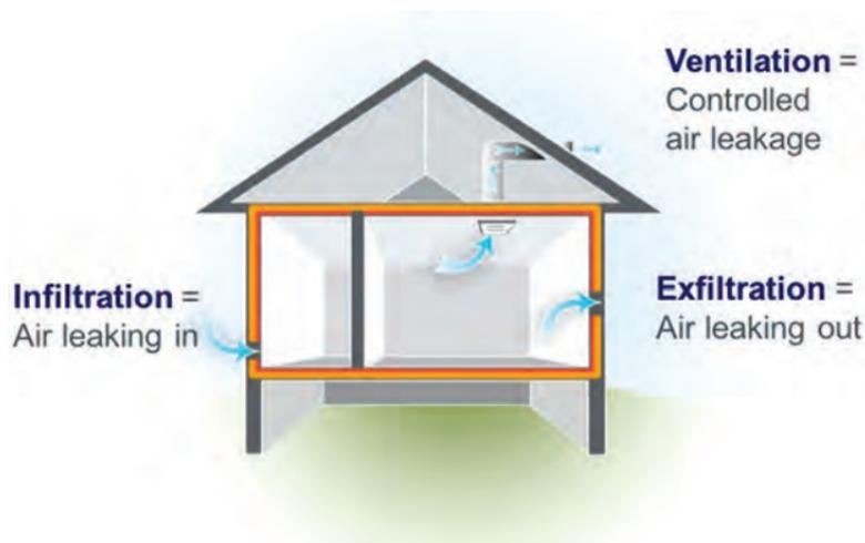
The air that leaks into the home through infiltration often comes from crawl spaces, attics, and building cavities. This air can carry mold, mildew, dust, radon, moisture, and other pollutants into the home. Air-sealing slows the flow of this unhealthy air. We often install ventilation systems in the bath and/or kitchen after doing air-sealing work so that stale air is removed from the home, and fresh air is supplied where and when we need it.
