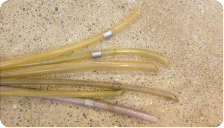
**You'll use flex tubes to fill the walls in most site-built homes.** To keep the job moving quickly, you want the fattest flex tubes that fit into the space you're insulating. Most crews carry 1" and 1¼" flex tubes. You should also carry different tubes for winter and summer—softer hoses will feed more easily in cold weather, but they will often kink when the weather is warm.
