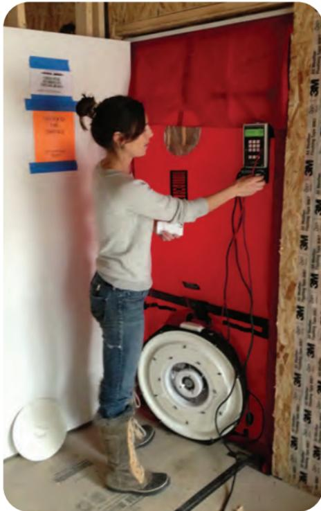
When you've completed the blower door test, return the home to the condition in which you found it, including turning any combustion appliances back to ON.
