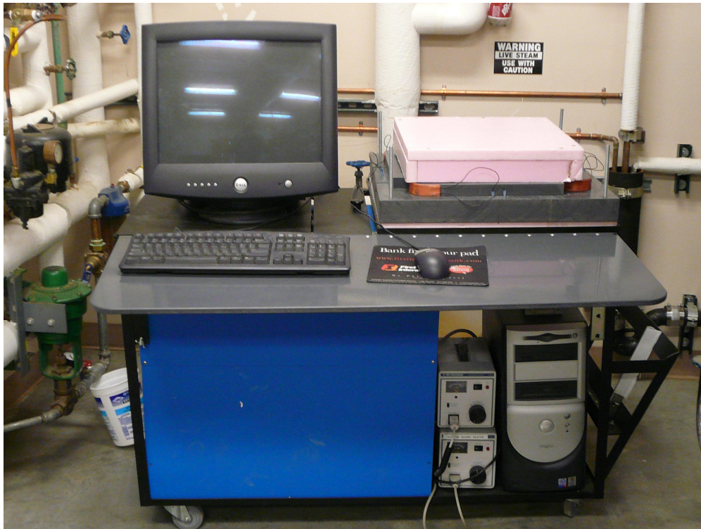
Figure 1: Thermal Conductivity Testing Apparatus
