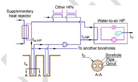
Figure 13: Schematic diagram of a closed- loop GSHP with vertical bore ground heat exchanger (Source: Sarbu and Sebarchievici 2013)
