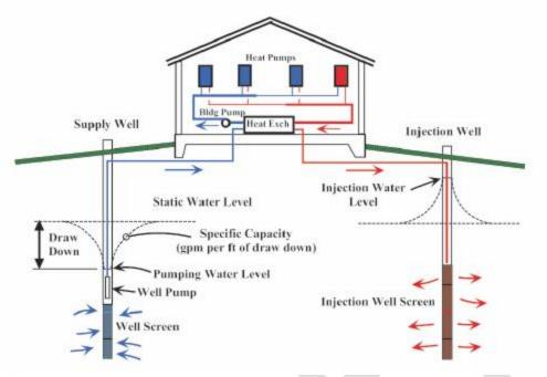
Figure 11: Schematic diagram of an open loop ground source heat pump with isolation heat exchanger (Source: Kavanaugh and Rafferty 2014)
