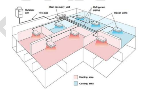
Figure 5: Schematic diagram of a VRF system
