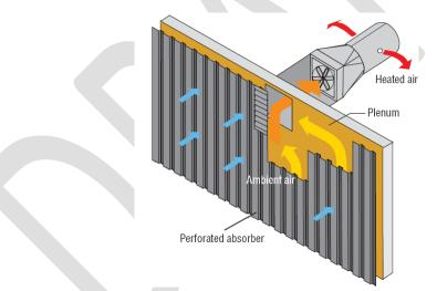
Figure 8: Schematic diagram of Transpired Solar Collector
