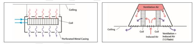
Figure 7: Schematic diagram of passive chilled beams (left) and active chilled beams (right)
