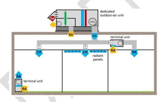
Figure 3: Diagram of a typical DOAS system
