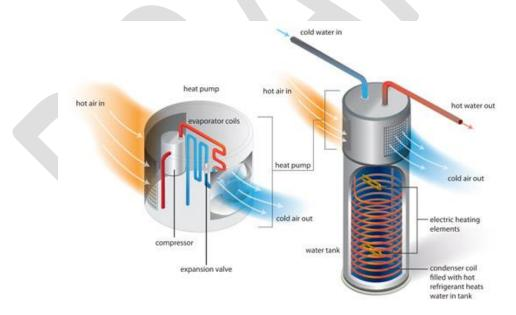
Figure 9: Schematic diagram of a Heat Pump Water Heater (Source: DOE ND)
