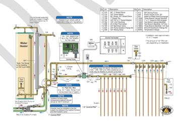
Figure 14: Schematic diagram of a radiant heating panel configuration (Source: Dasmu.us)
