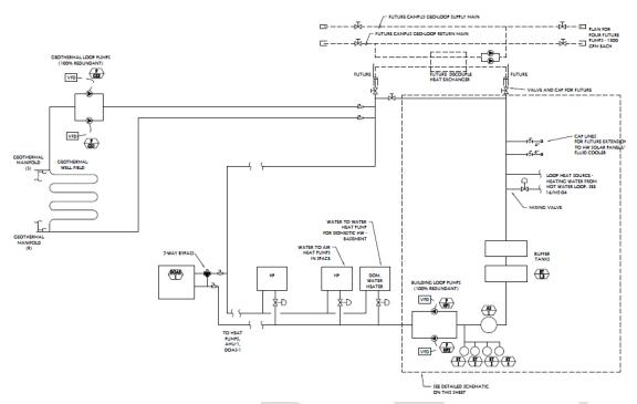
Figure C-10: Norm Asbjornson Innovation Hall heat pump loop schematic
