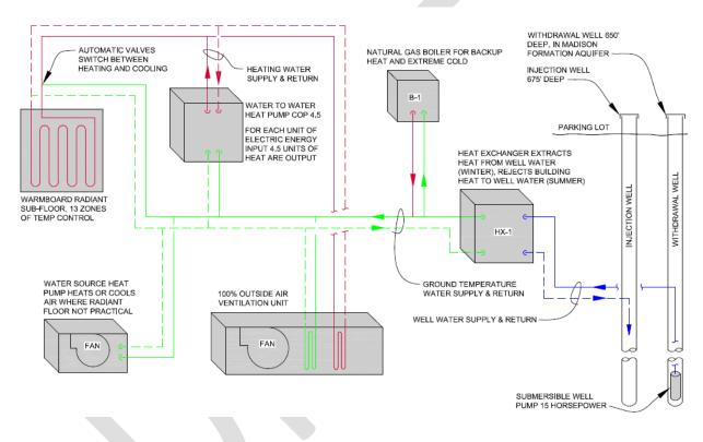
Figure C-4: Conceptual diagram of mechanical systems for the CTA office, Great Falls Montana
