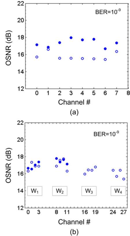
Fig. 6. OSNR (measured in a resolution bandwidth  $RB = 0.08$  nm) required for  $BER = 10^{-9}$  for all channels: (a) original and (b) optimized optical interconnect architecture. (Symbols:  $W_1 - W_4$ : wavebands used in the optimized architecture; Open and filled circles: simulated and experimental results, respectively).
