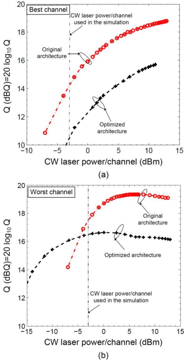
Fig. 8. Q-factor versus CW laser power (a) for the best and (b) for the worst channel of both the original and the optimized architecture. (Symbols: Red dashed line with circles: WDM transmission in the original architecture, Black dashed line with crosses: WDM transmission in the optimized architecture).
