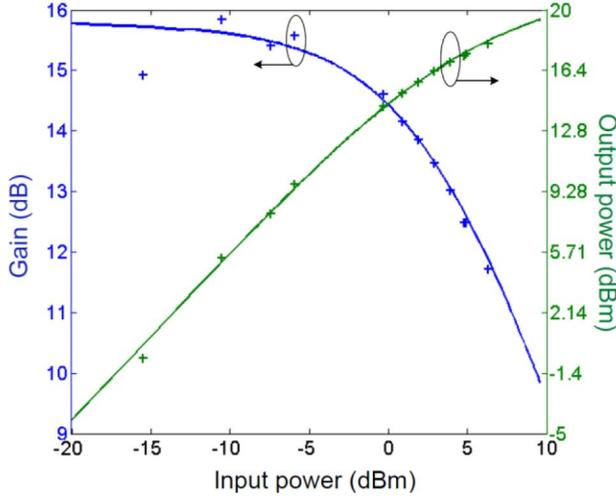
Fig. 9. Fitting experimental data for the SOA gain (blue) and for the output power (green) as a function of input power using the TLM simulation model. (Symbols:  $P_{in}$  = Input SOA power,  $P_{out}$  = Output SOA power, Solid line: Simulation, Crosses: Experimental values).
