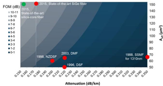
Fig. 1. FOM with respect to 0.350 dB/km fiber with  $A_{\text{eff}} = 67 \mu\text{m}^2$  in a 65 km span configuration.
