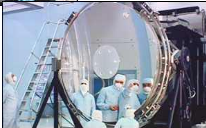
COSTAR corrective optics installed in 1993
