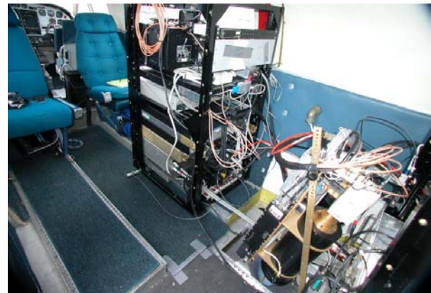
Figure 2. Lidar inside the airplane in September 2004. From left to right are backward-facing seats for lidar operator and observer, lidar electronics rack, and the lidar optics head looking through a hole in the airplane floor. (J. Shaw photo).
