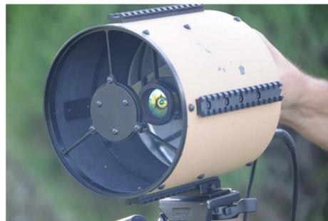
Fig. 3. Telescope-mounted LWIR camera used for observing IR mirages.
