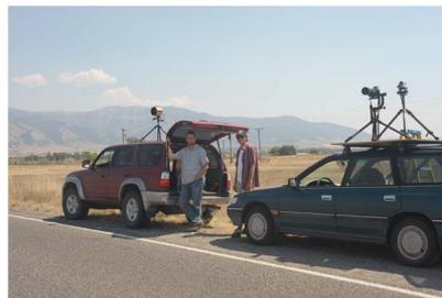
Fig. 4. Airport mirage imaging experiment in August 2012 with an IR camera (left) and VIS cameras (right).
