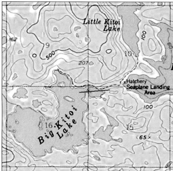
Fig. 12. King Air west-to-east flight track at 160-m height over a bay in the northeast end of Big Kitoi Lake on Afognak Island in Alaska. The flight line is in the center of the figure, and the superimposed grid is in statute miles. The map was generated with National Geographic TOPO! software, and the elevations and depths are in feet.
