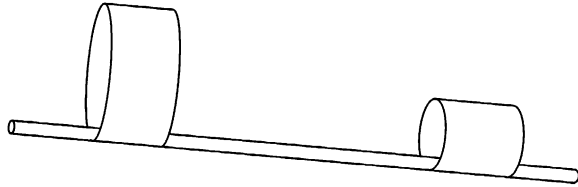
FIGURE 1.—Straw glider paper airplane used in this lab. Each “wing” is made of a strip of paper taped in a circle to the straw “fuselage.”
