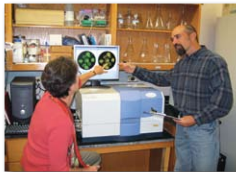
Lab Manager Susan Broadway (left) and statistician Albert Parker with the ScanRDI solid phase laser cytometer. Photo courtesy of Steve Hammer
