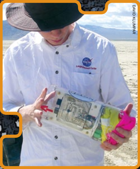
While testing the satellite, MSU graduate Scotty Kratochvil checks a parachute packed inside a canister that holds the MSU instrument.
